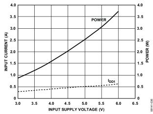
Figure 16. Typical Short-Circuit Input Current and Power vs. V<sub>DD1</sub> Supply Voltage
