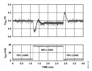
Figure 17. Typical  $V_{\rm ISO}$  Transient Load Response, 5 V Output, 10% to 90% Load Step
