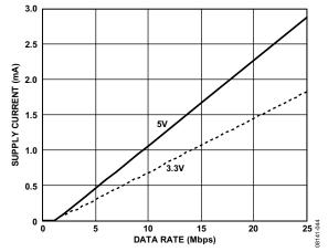
Figure 26. Typical I<sub>ISO(D)</sub> Dynamic Supply Current per Output (15 pF Output Load)
