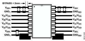
Figure 27. Recommended PCB Layout
