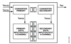
Figure 31. Power Consumption Within the ADuM640x
