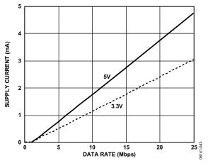
Figure 25. Typical I<sub>ISO(D)</sub> Dynamic Supply Current per Input
