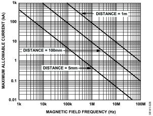
Figure 30. Maximum Allowable Current for Various Current-to-ADuM640x Spacings
