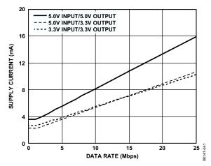
Figure 23. Typical I<sub>CHn</sub> Supply Current per Forward Data Channel (15 pF Output Load)
