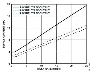
Figure 24. Typical I<sub>CHn</sub> Supply Current per Reverse Data Channel (15 pF Output Load)
