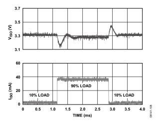
Figure 18. Typical  $V_{\rm ISO}$  Transient Load Response, 3.3 V Output, 10% to 90% Load Step
