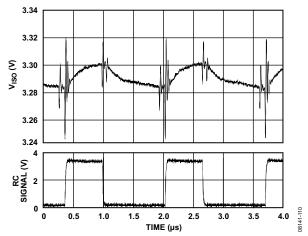
Figure 20. Typical Output Voltage Ripple at 90% Load, V<sub>ISO</sub> = 3.3 V
