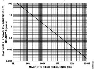
Figure 29. Maximum Allowable External Magnetic Flux Density
